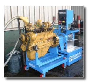
With the engine in position, the flywheel connected to a guarded universal joint drive shaft with just a few bolts. Through the use of the drive shaft and the guided positioning of the engine on the cart, time spent connecting the engine is minimal.
